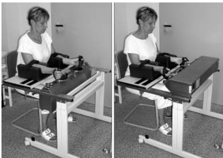
Fig. 6. The computer-assisted arm trainer Bi-Manu-Track for hemiparetic patients with a severe upper limb paresis.
